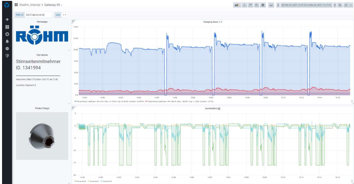
Figure 7: Manufacturing of face driver plates. The iJaw measures the clamping force at 100 Hz during machining in real time. The data is forwarded to the gateway and from there to the machine control system and/or a cloud.
