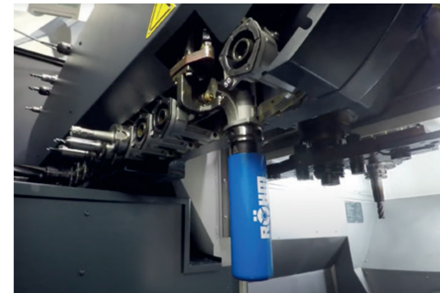
The Lubritool has its fixed place in the tool changer and is simply swapped in cyclically by the machining program
