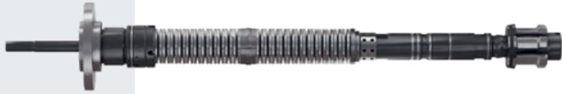
The HSK-FLEX is a tool clamp for automatic clamping machines with a spindle drive. It is installed directly into the machine tool spindle, i.e. into the rotor of the drive motor, which is designed as a hollow shaft for this purpose. Designed in particular for milling machines that operate at high speeds, it is equipped with the HSK tool holder clamping head.
