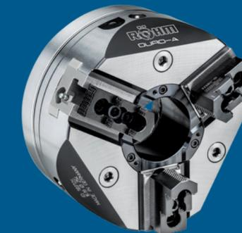
sleeve (3) seals the chuck and protects it from chips. The threaded ring (4) ensures a stable connection with the cylinder. Röhm also offers a threaded blank (draw tube adapter). Here, the unit uses fitted adapter rings to connect to a machine shaft with a short cone. The base jaws (6) are optionally equipped with a teeth serration of 60° or 90°.
