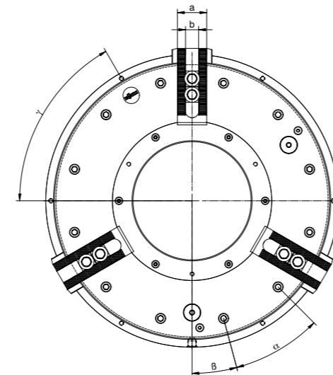
**LVE** - large through-hole, with pressure control device, rapid and clamping jaw movement
