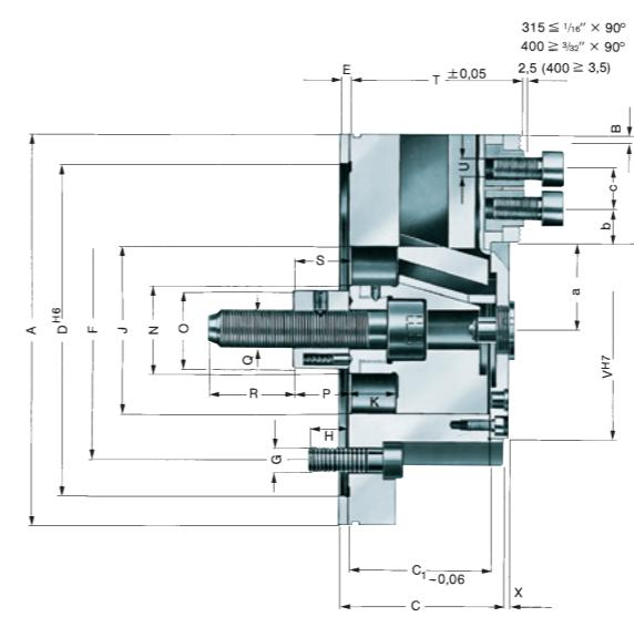
**2-jaw power chuck, weight reduced, serration 90°**
