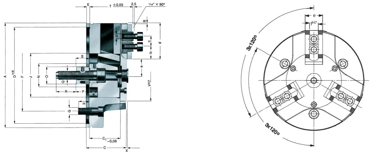
**3-jaw power chuck, weight reduced, serration 90°**
