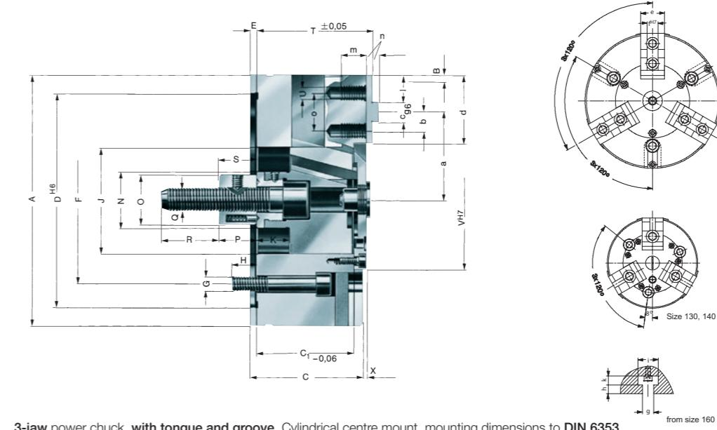
3-jaw power chuck, with tongue and groove, Cylindrical centre mount, mounting dimensions to DIN 6353
