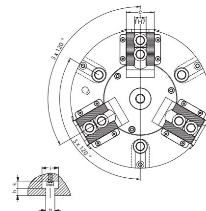
Low maintenance 3-jaw power chuck KFD-EC, with short piston, without force compensation, centric clamping cylindrical centre mount, mounting dimensions to DIN 6353
