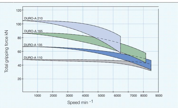
To obtain the specified gripping forces, the chuck must be in a perfect condition and lubricated with F 80 lubricant recommended by RÖHM. Measuring point near chuck face.
