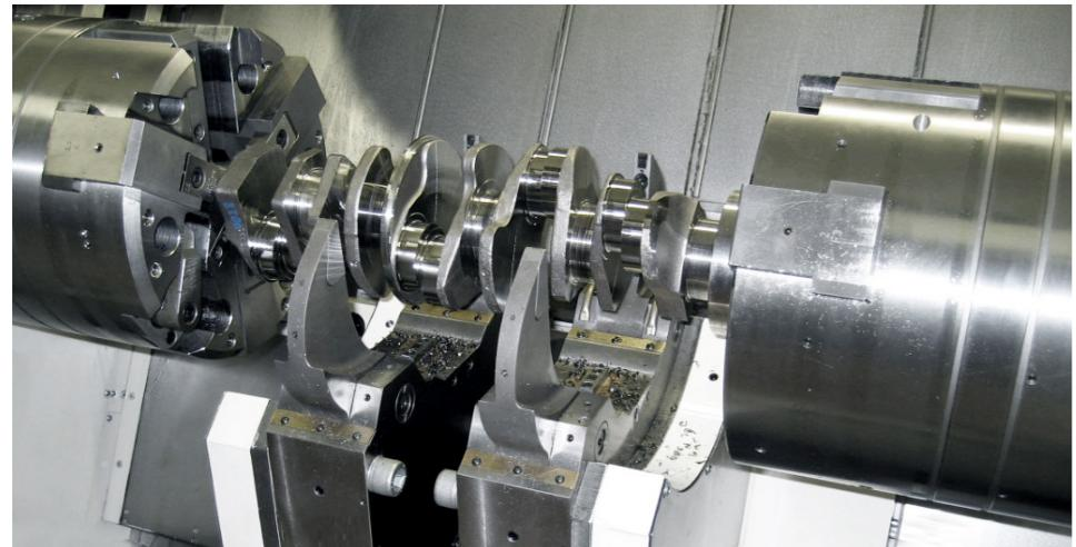
Optimal support of components for every application, e.g. crankshaft machining
