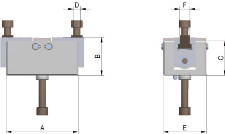
2-jaw gripper chucks **GF** for cylindrical shank DIN 69880, chucks without shank, without jaws
