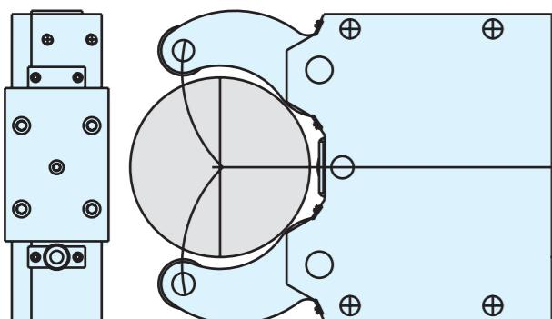
All steady rests of type SLZN and SLZNB can be equipped with holders and rods or only with rods, in order to be able to control the clamping position and open position using limit switches.
