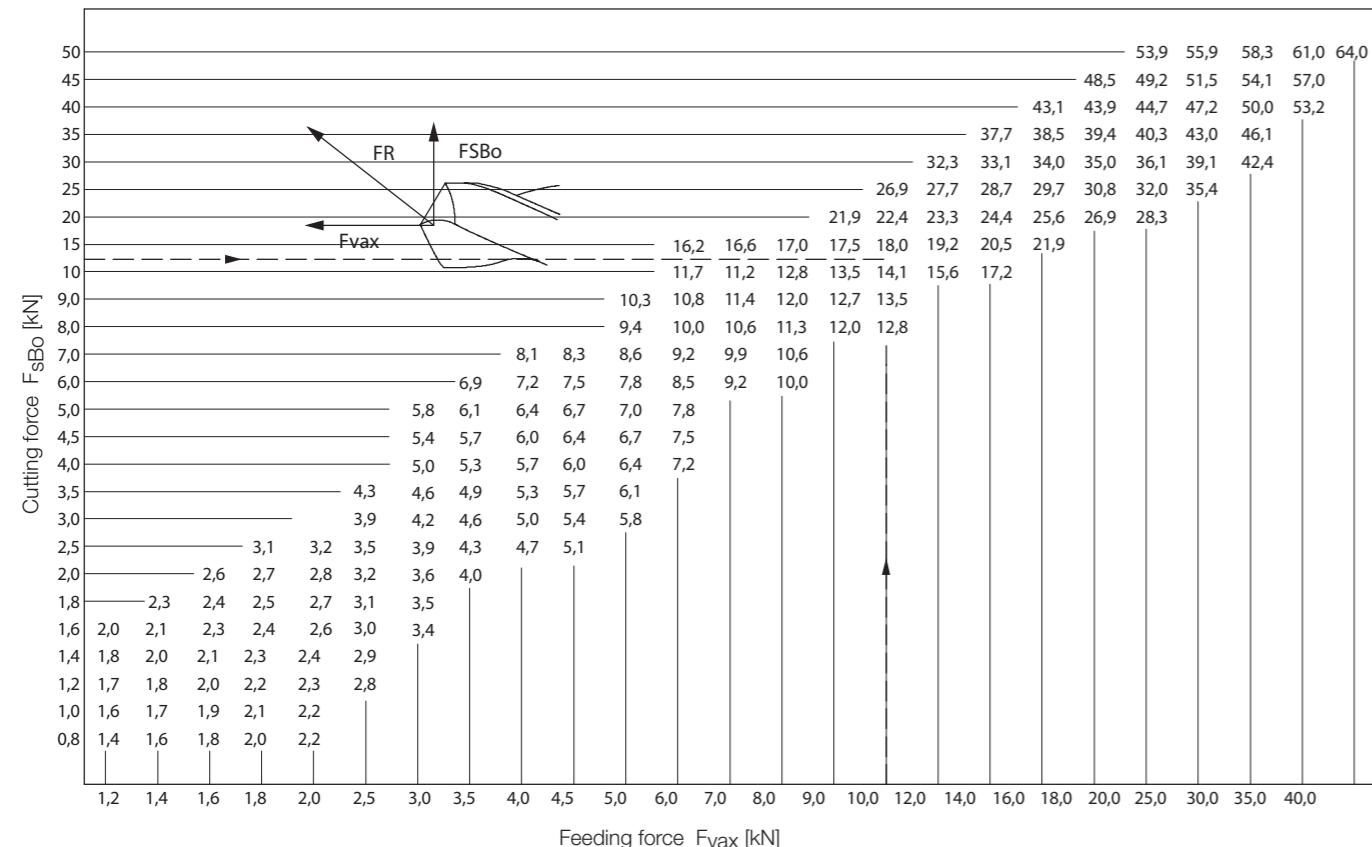
Place resultant force  $F_R$  for drilling in solid material in the known formula for determining the required gripping force  $F_{spz}$ :
