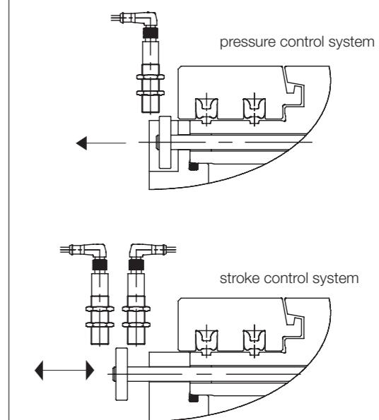
The control unit is designed for LVE chucks with rapid and clamping strokes only for external clamping. For LVE chucks with a normal stroke only pressure control device for the external clamping is provided (on customer demand for internal clamping).
