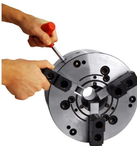
The quick jaw change system allows flexible use of the power chuck and drastically reduces set-up times. The jaws can be flexibly offset, turned or changed.
