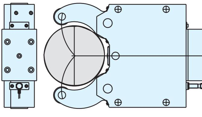
There is the option of attaching a sensor (proximity switch) to the steady rests as standard, which measures the position of the opened steady rest. This option is not available for the steady rest of type SLZ-047. The proximity switch is not included in the delivery of the steady rest.
