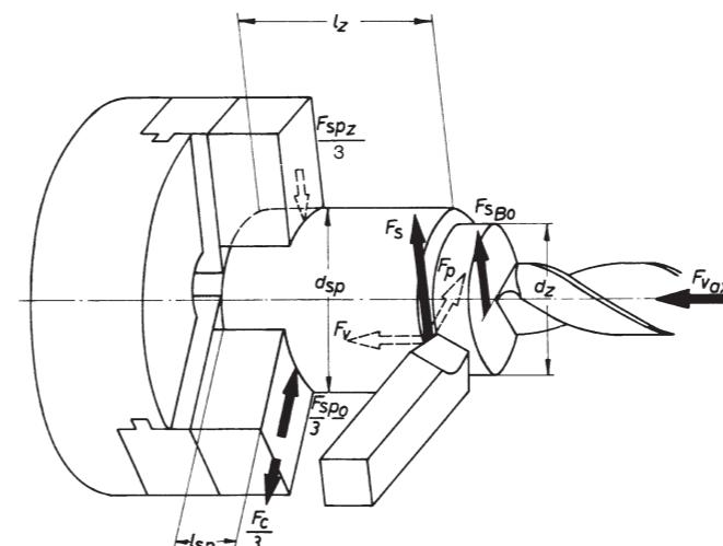
**F<sub>s</sub>** = Main cutting force on radially applied tool
