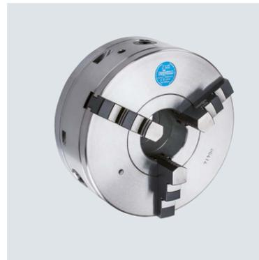
*In contrast with the Hi-Tru, in the ES version the 3 or 4 clamping jaws can be adjusted individually to each other, thus allowing adaptation to the clamping geometry (e.g. cast components). This means that a defined positioning of the workpiece in relation to the chuck's center of rotation is possible.*
