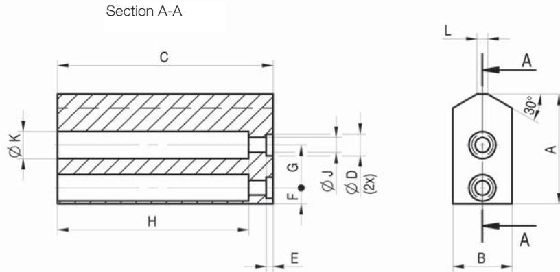
Jaw blank - steel (including fixing screws)
