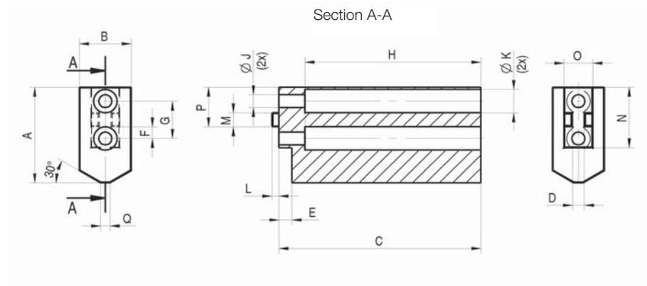
Jaw blank - steel (including fixing screws)
