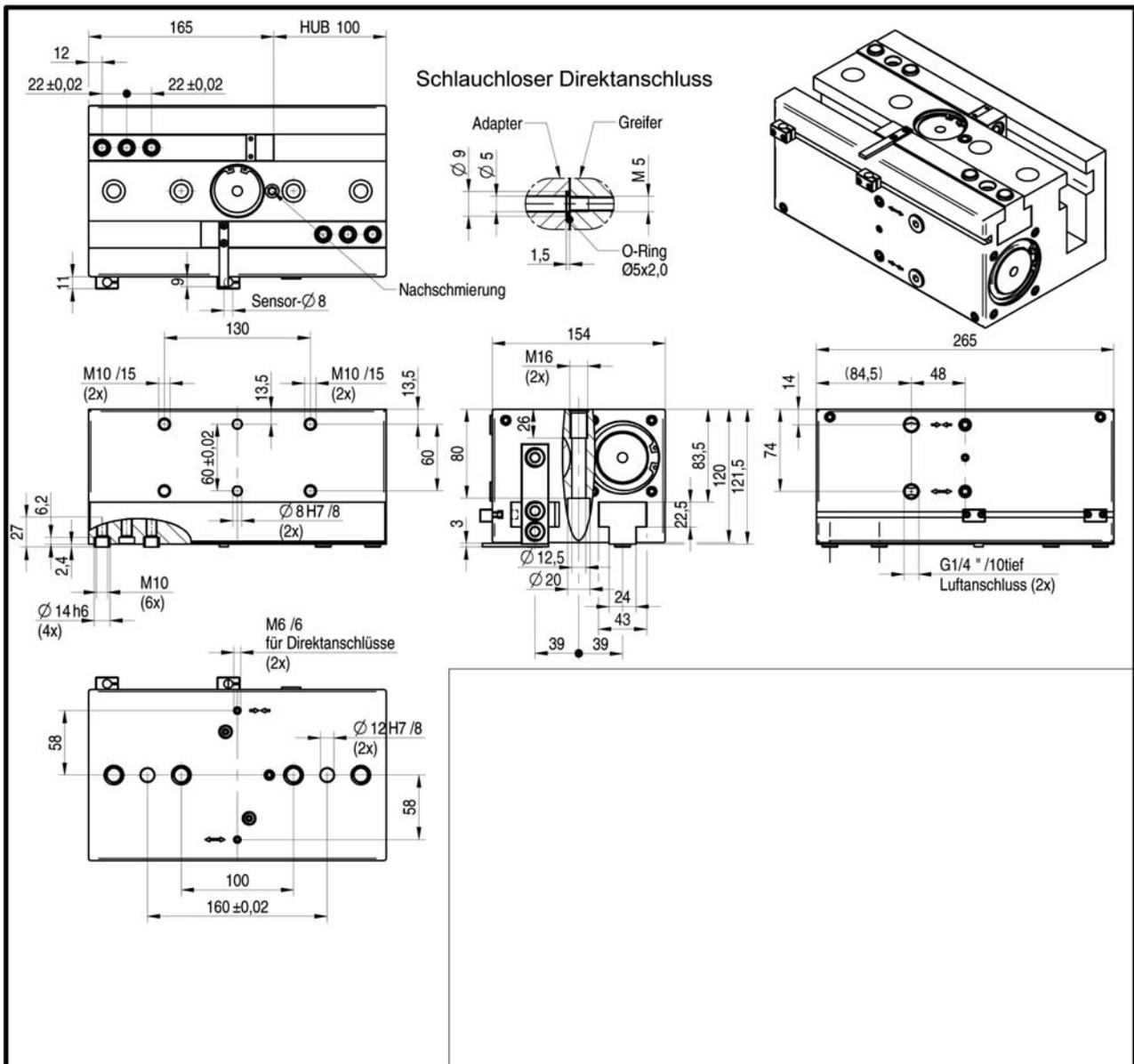
2-jaw long stroke gripper
