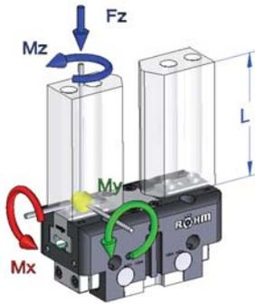
Clamping force diagram exterior gripping
