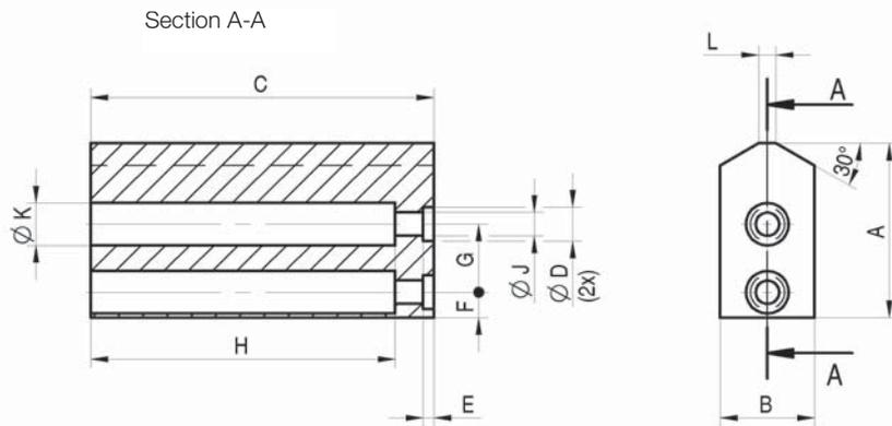
**Jaw blank - aluminium** (including fixing screws)
