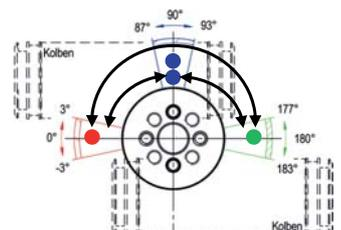
with mechanically locked middle position
