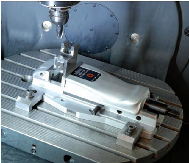
The RÖHM machine vice is suitable for universal application on milling machines and machining centers. The base is equipped with grooves to ensure a precise fastening on the machine table.
