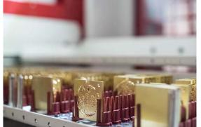
Bild Nr. 35-01 RM\_IW-Platinen.jpg The manufacturing of the watch plate at IWC brings the manufacture calibre to birth. © Benedict Walther für Röhm
