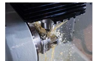
Bild Nr. 35-04 RM\_IW-Fertigung.jpg The prizewinning power index chuck from RÖHM supports machining from three sides with just one clamping position.
