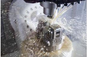
Bild Nr. 35-06 RM\_IW-AufzugswelleBohrung.jpg IWC carries out all the necessary operations (milling, drilling, thread cutting, piercing and the fine machining of the edges) in just one clamping position. © Benedict Walther für Röhm
