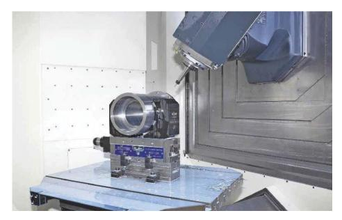
Despite the very big overhang of around 284 millimetres, Röhm can guarantee repeatability of one-hundredth of a millimetre and a clamping force of four tons with the NC-Compact centric vice of the RKZ series.
