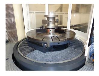
This DURO-TA XT chucks from Röhm with an impressive 1200 mm diameter are characterised by their compact design, workpiece accessibility, flexibility and clamping force despite their size.
