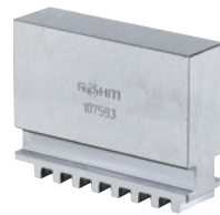
A09 Unstepped jaw BL, DIN 6350, unstepped, soft, material 16MnCr5
