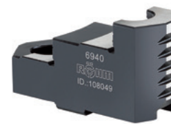
A09 Reversible top jaws UB, DIN 6350, hardened tongue and groove for external and internal clamping, material 16 MnCr5
