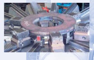
Power operated wedge chuck KFD, dia. 2800/6
