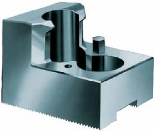
Tool group C 21 Type 543-33 Claw-type jaws , 1 piece, hardened, serration 60° - width of the groove 12
