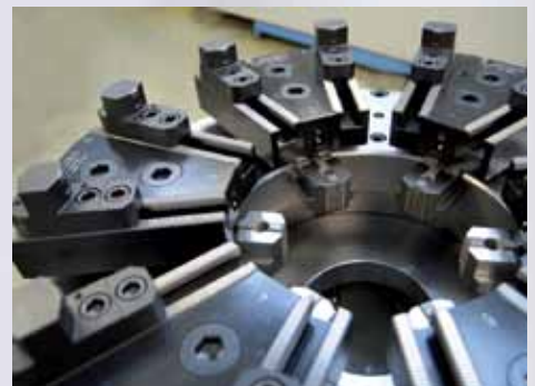
Variable positioning of the clamping jaws on the pedulum segments
