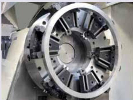
For clamping thin walled workpieces
