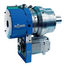
Electrical cylinder EHS for actuating chucks with through-hole. Especially suitable for clamping bars with an outside diameter of up to 67 mm on lathes and grinding machines.
