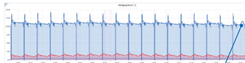
Clamping force measurement (left) in series production. Production of 18 drive plates (right). The clamping force progression is like the fingerprint of the manufacturing step. Significant variations are an indication of faults and thus of incorrect production and a faulty product.
