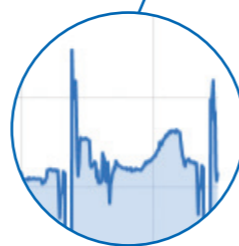
Clamping force measurement (left) in series production. Production of 18 drive plates (right). The clamping force progression is like the fingerprint of the manufacturing step. Significant variations are an indication of faults and thus of incorrect production and a faulty product.
