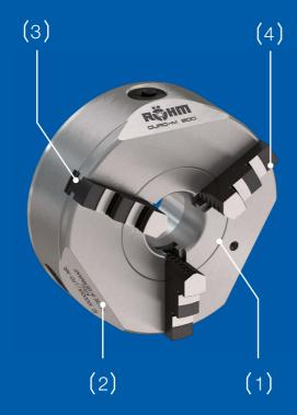
Due to the principle (including manufacturing tolerances) there is one drive that is more precise than the others. This so-called "zero drive" is identified during manufacture of the chuck by RÖHM and is clearly indicated by an arrow. The first time the jaws are finish ground (also during manufacturing by RÖHM), this drive is used for clamping.
