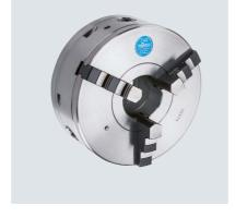
In contrast with the Hi-Tru, in the ES version the 3 or 4 clamping jaws can be adjusted individually to each other, thus allowing adaptation to the clamping geometry (e.g. cast components). This means that a defined positioning of the workpiece in relation to the chuck's center of rotation is possible.
