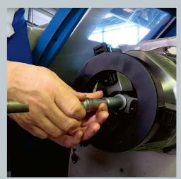
**5.** Loosen the jaw cutting attachment
