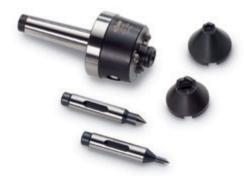
consisting of 1x base body, 2x driver discs (clamping diameter 12, 32), 2x center points (centering Ø 6, 16)
