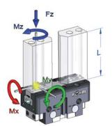
Clamping force diagram exterior gripping
