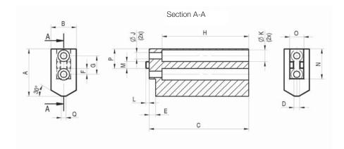
Jaw blank - aluminium (including fixing screws
