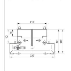
Type GA/GI with gripping force safety device
