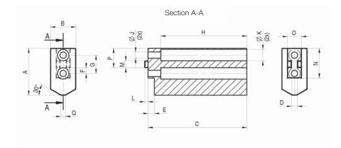
Jaw blank - steel (including fixing screws)
