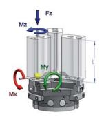
Clamping force diagram exterior gripping
