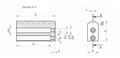
Jaw blank - aluminium (including fixing screws)
