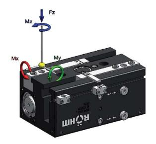
Clamping force diagram exterior gripping
