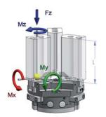
Clamping force diagram exterior gripping
