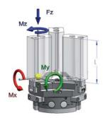
Clamping force diagram exterior gripping
