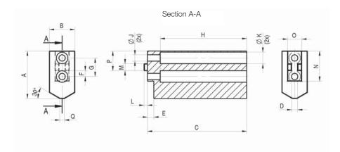
Jaw blank - steel (including fixing screws)
