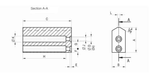
Jaw blank - aluminium (including fixing screws)
