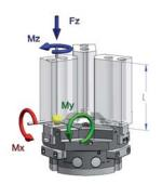
Clamping force diagram exterior gripping
