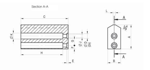
Jaw blank - steel (including fixing screws)
