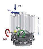
Clamping force diagram exterior gripping
