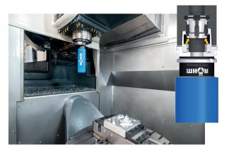
The lubrication impulse is automatically activated within the spindle. An optimal quantity of Lubriflux lubricant is sprayed onto the right place of the tool clamping system.
